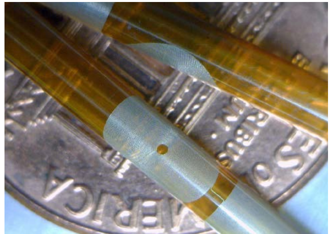
Figure 3: Medical device fabricated in polyimide tubing with 10 micron vias and traces that have been filled with silver nanoparticle conductive material.
